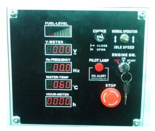
QYCB-1 model gasoline genset control panel that is set in the genset'box is designed for the manual operation gasoline genset. It has the start swith, the emergency stop swith, the idle swith, the choke swith, the engine oil alert pilot lamp. The display LED circuit board can display the Fuel-level, Voltage, Frequency, water temperature, operating time.
